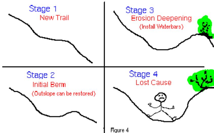
down the centerline of the trail (Stage 3). If this centerline gullying is allowed to continue unchecked, the trail will trench deeper and deeper until it is both unusable and unredeemable (Stage 4).
