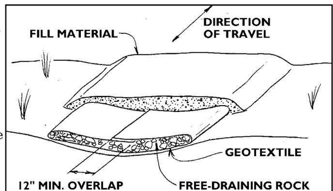
The rock may be single size material from pea gravel to cobbles (3-12") or a mixture of rock material that does not contain silt or clay. The free-draining rock can be placed to a thickness equal to the largest rock if only drainage is desired. If reinforcement is also needed, at least 3" of rock is recommended. The geotextile is wrapped over the rock layer with a 12" overlap to ensure encapsulation, since settlement of saturated soil can pull the overlap joint apart.
