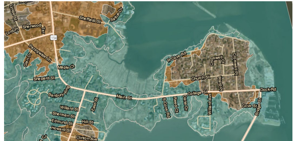
Figure 5-5: Limits of FEMA Special Flood Hazard Area around Route 154
