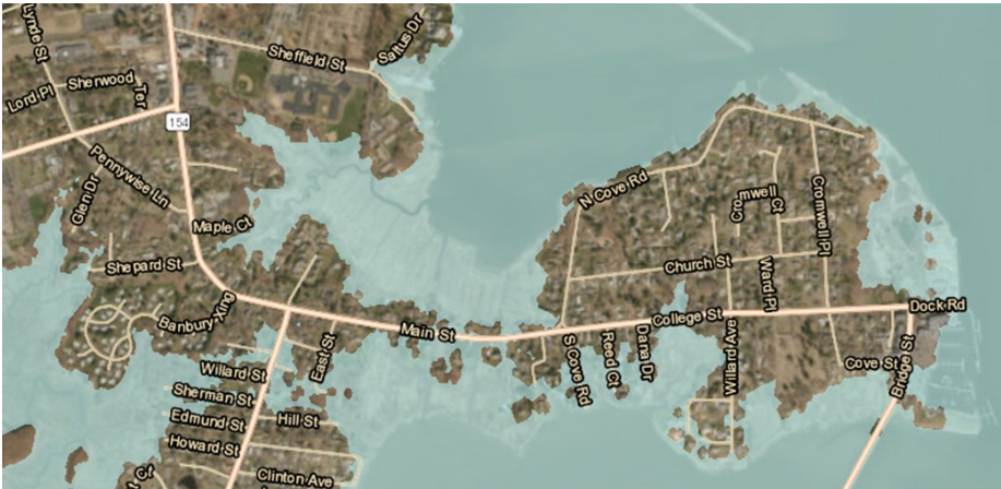
Figure 5-7: Limits of 10-year Recurrence Interval Flood around Route 154
