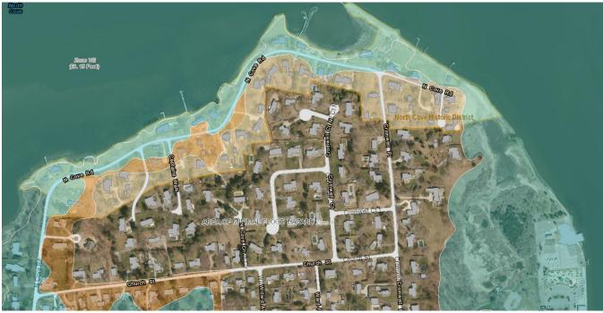
Figure 4-29 The North Cove Historic District relative to FEMA Special Flood Hazard Zones Note: Areas shaded in green represents the FEMA AE zone and areas in brown are located within the limits of the 500-year recurrence interval flood.
