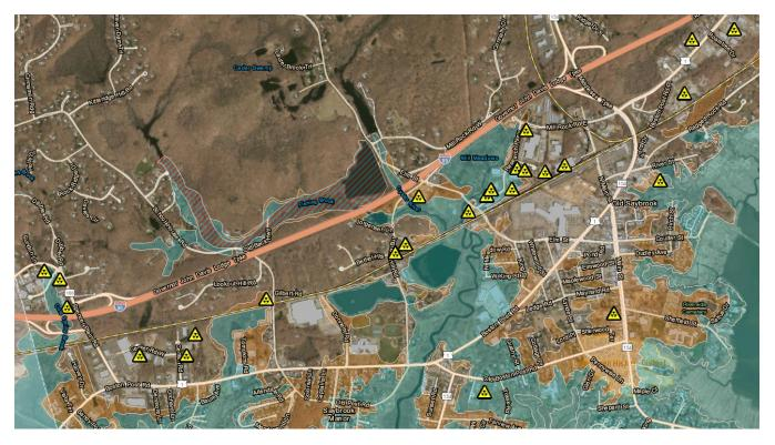
Figure 4-32 Old Saybrook Hazardous Materials Facilities relative to FEMA Special Flood Hazard Zones Note: FEMA AE zone limits shown in green and FEMA 500-year recurrence interval flood limits shown in brown.
