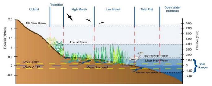
Figure 4-55: Relationship between Tides, Wetlands and Reference Elevations for Typical Connecticut Estuarine Marsh Profiles
