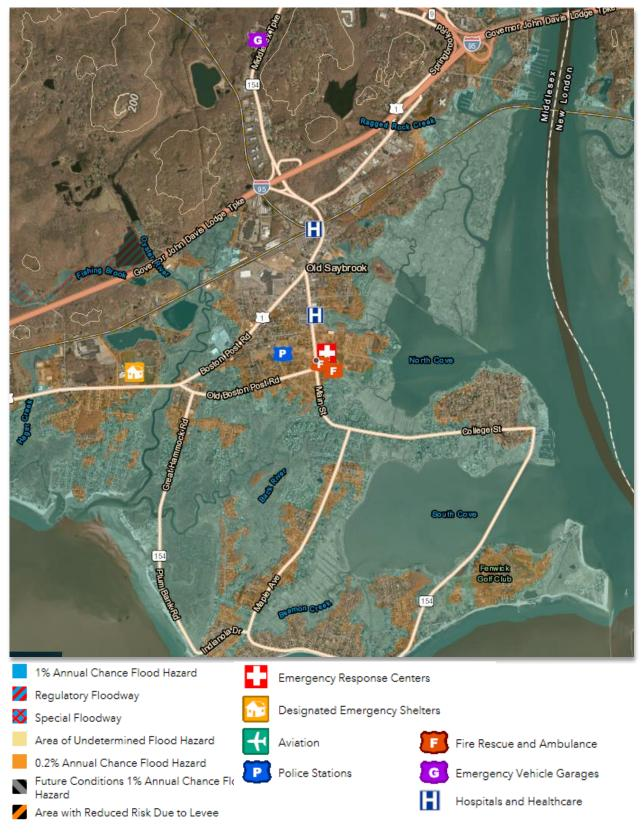
Figure 4-18 Location of Essential Facilities relative to Predicted Coastal Flood Limits FEMA FIRM Note: Areas shaded in green represents the FEMA AE zone and areas in brown are located within the limits of the 500-year recurrence interval flood.
