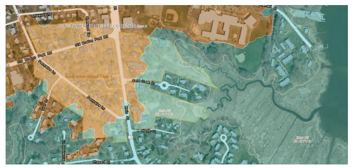
Figure 4-30 The South Green Historic District relative to FEMA Special Flood Hazard Zones Note: Areas shaded in green represents the FEMA AE zone and areas in brown are located within the limits of the 500-year recurrence interval flood.
