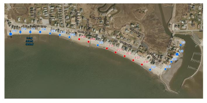
This stretch of shoreline is characterized by artificial fill placed within the marsh and estuarine beach deposits, with the beach characterized as a barrier spit. The shoreline is fortified with groins and sea walls. The upland ground surface elevation is about 4 to 6 feet NAVD88.
