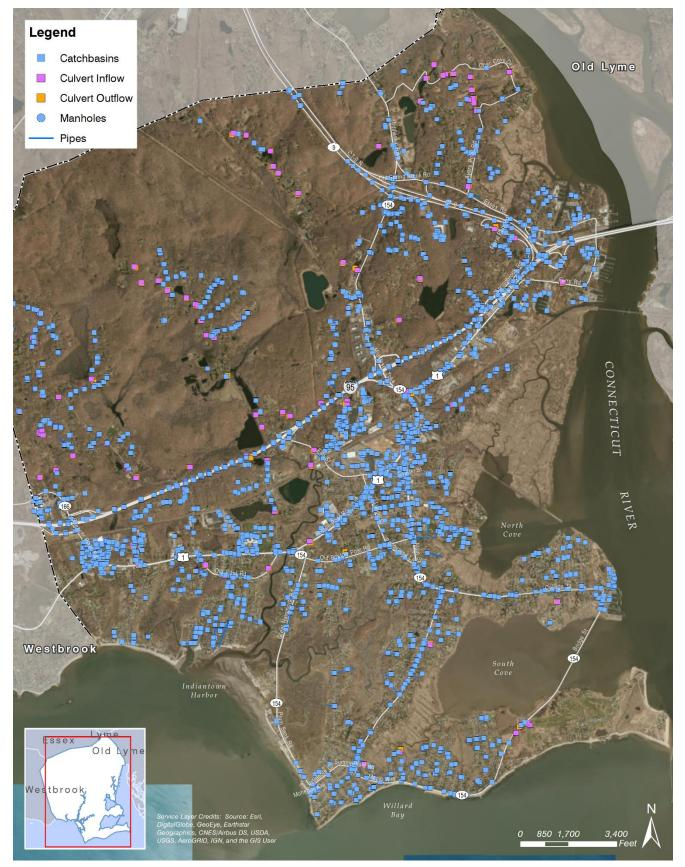
Figure 4-51: Stormwater Catch Basins and Culvert Inflows/Outflows
