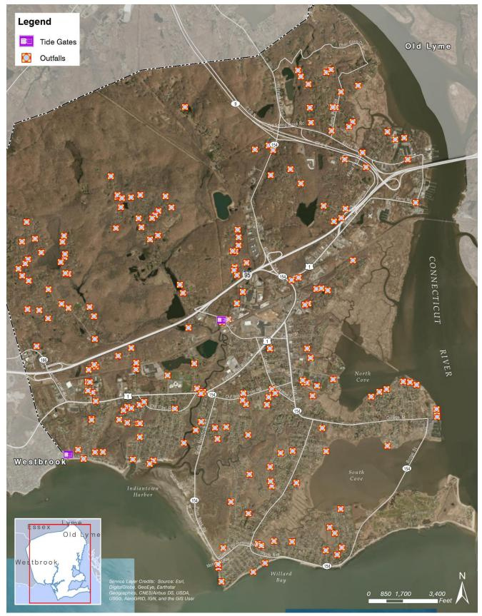
Figure 4-52: Stormwater Outfalls and Tide Gates
