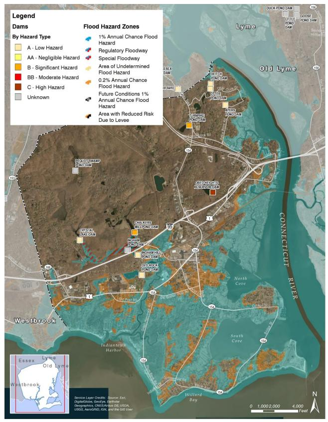
Figure 4-28 Location of Old Saybrook Dams relative to FEMA Special Flood Hazard Zones. Note: Areas shaded in green represents the FEMA AE zone and areas in brown are located within the limits of the 500-year recurrence interval flood.
