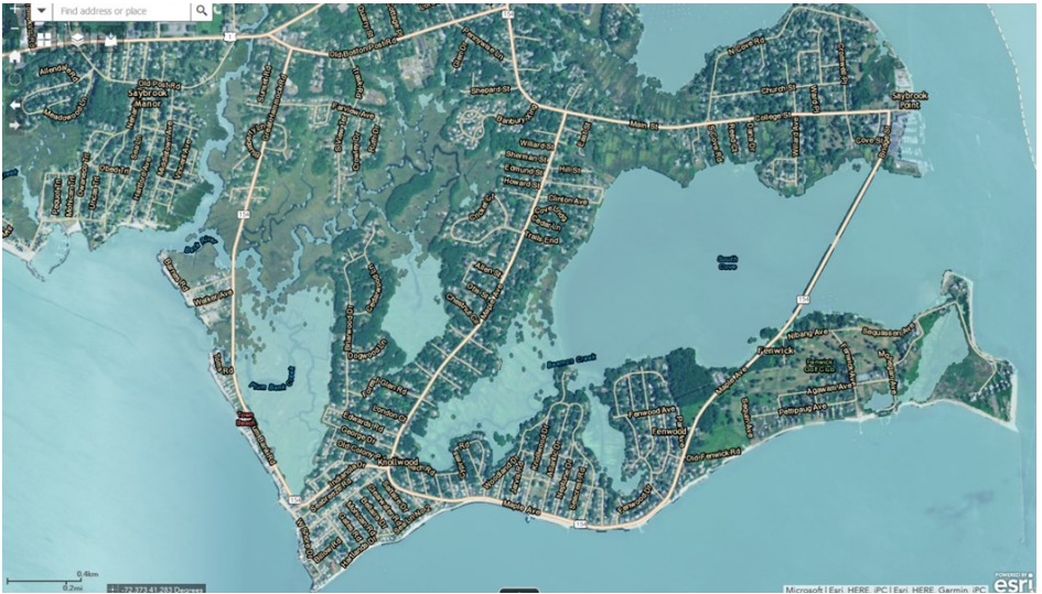
Figure 2-8: Predicted MHW Flood Inundation by the year 2066 assuming USACE Intermediate Sea Level Rise Projection
